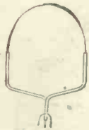
Here we have the arch-shaped filament. Note how securely it is welded to stout electrodes. Its very shape prevents it from falling or sagging—a fruitful cause of breakdown in other types of Valves.
